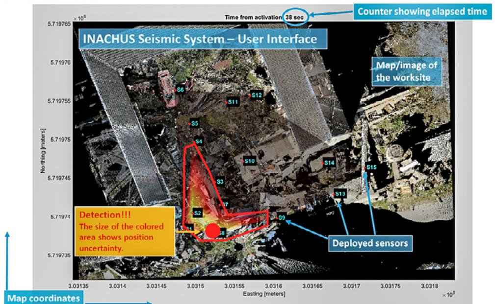
At Pilot 3, the GBSS was deployed on a rubble pile to detect and locate a person acting as a victim in the tunnels underneath the debris. A large power generator was placed on a concrete slab on the rubble to test and demonstrate the system’s ability to detect signals even in the presence of very strong background noise.
