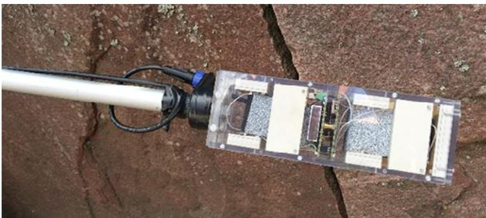
The INACHUS Robot and the RobotRadar were developed during the same period and a mock-up for the robot was needed to be able to test the radar before the robot was available. This special test-platform was further developed to a new product, the StickRadar. It consists of the same radar system as in the RobotRadar, but instead of a robot it is mounted on a telescopic stick and it will
